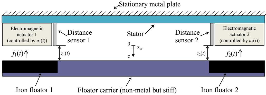
Fig. 1. Sectional view of the magnetic suspension system.
